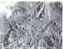
One-component cement-based waterproofing slurry
